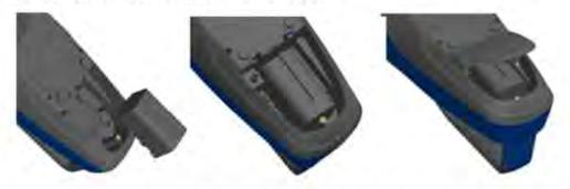
Figure 2-2: Batteries into Handheld Unit
