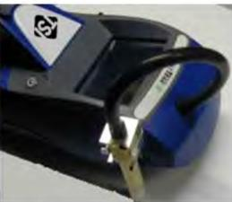
Figure 2-8: Installing Door-Oliver Cyclone
