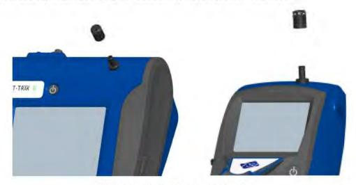
Figure 2-6: Putting on Inlet Cap
