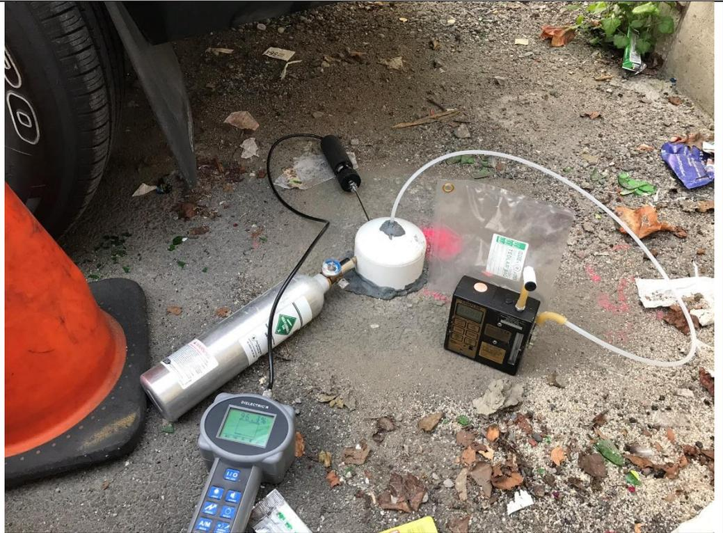
Photo 2 – Collection of LSV-14 soil vapor sample, facing west.
