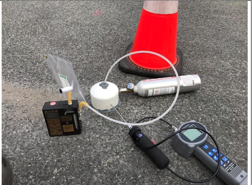
Photo 1 – Helium testing at LSV-18, facing south.
