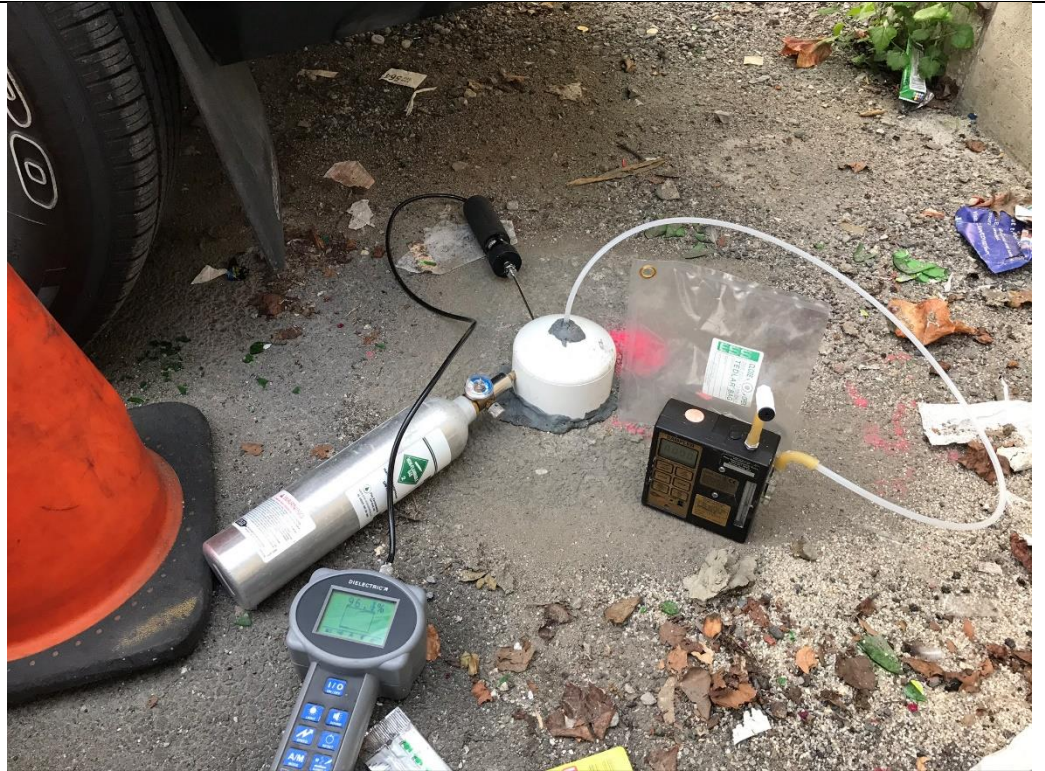
Photo 1 – Helium testing at LSV-15, facing south.
