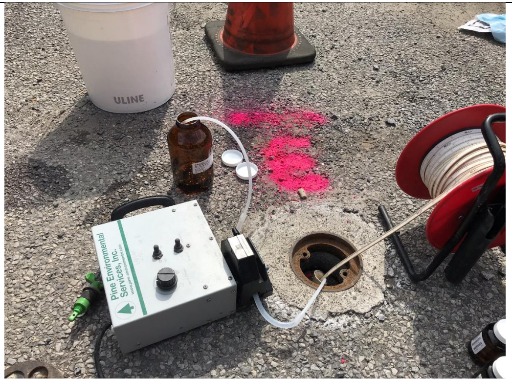
Photo 2 – Collection of groundwater sample at LMW-3, facing southeast.
