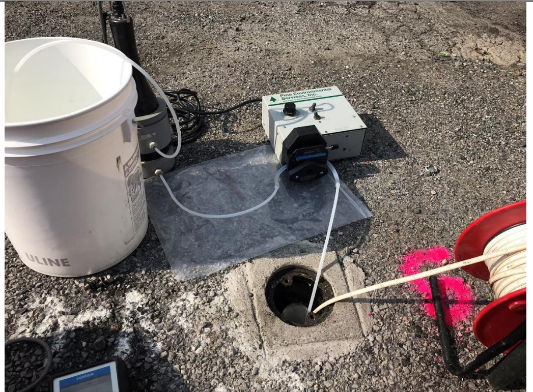
Photo 1 – Low flow groundwater purging at LMW-9, facing south.
