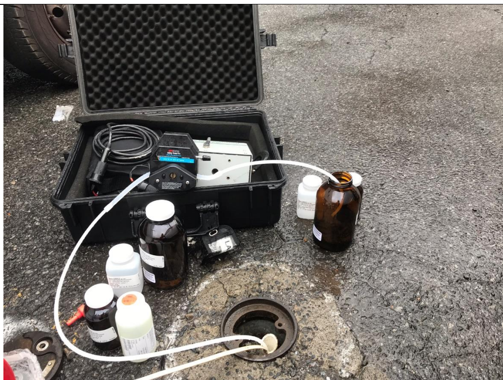
Photo 2 – Collection of groundwater sample at LMW-1, facing south.
