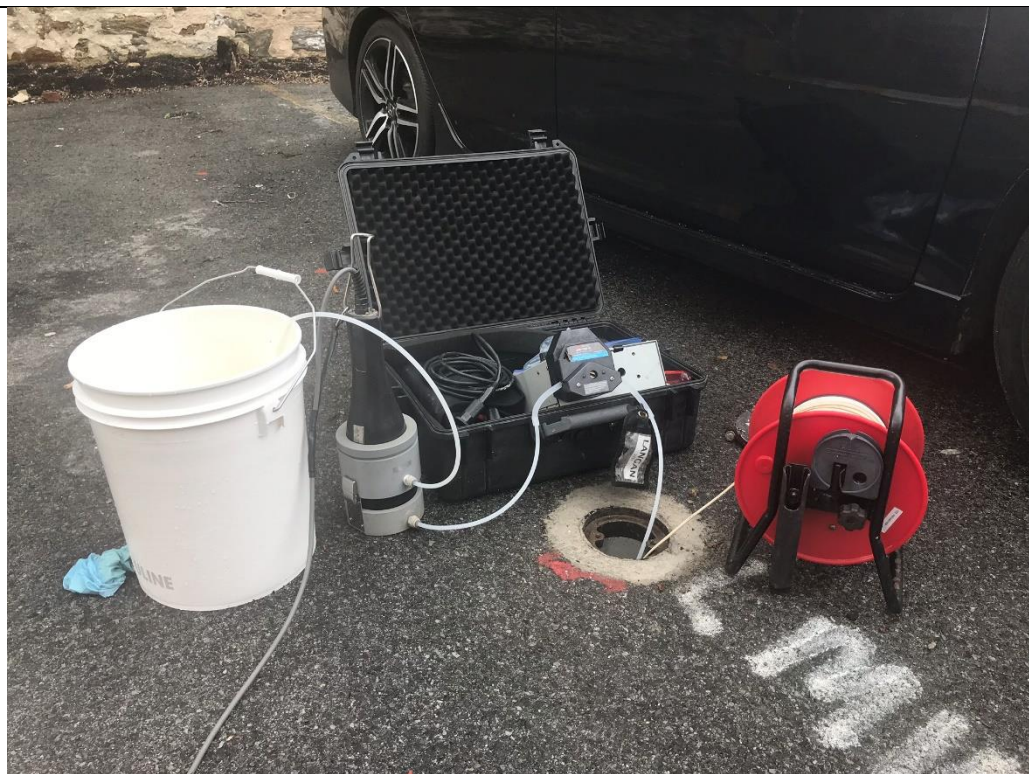
Photo 1 – Low flow groundwater purging at LMW-7, facing south.
