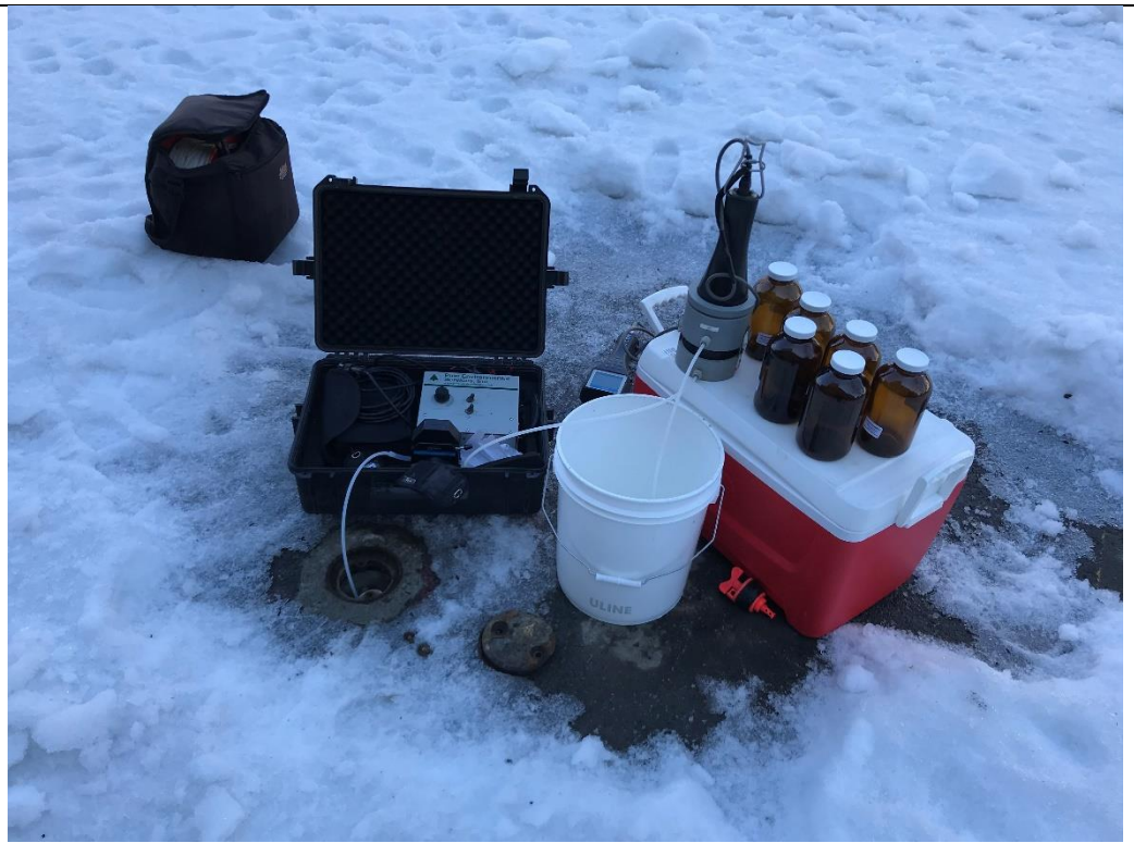
Photo 2 – Groundwater low flow purging at LMW-7, facing north.
